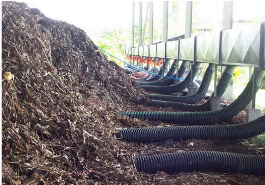
Industrial Scale Composting: Blowers assure an aerobic process that reduces greenhouse gasses
